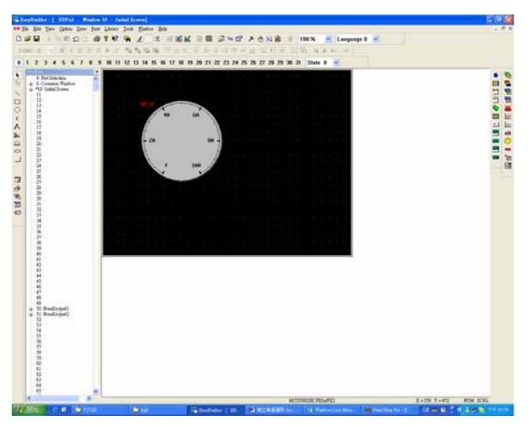
5. Adding Meter Display object, adjust bitmap and meter size to be the same size and position, and then save to Group Library.
